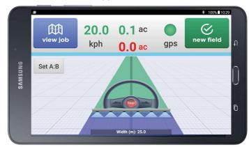
4. A-B lines are automatically set against the current heading, and can be reset to current heading whenever needed.
